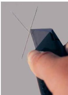
To perform this test a utility knife is used to make two cuts into the coating to form an “X”. At the vertex, the point of the knife is used to attempt to lift up the coating from the substrate. The evaluation of adhesion is based on both the degree of difficulty to remove the coating from the substrate and the size of removed coating. ASTM D6677 is the standard for this test method.
