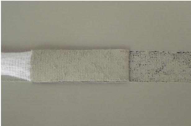
Figure 3 - Cohesive Failure
