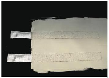
Figure 1 - Polyester Test Strips embedded into coating.
