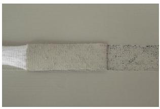
Figure 3 - Cohesive Failure
