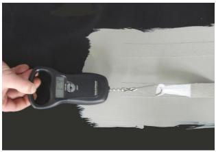
Figure 2 - Digital scale used to evaluate adhesion
